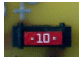
Battery Pack Fuse
